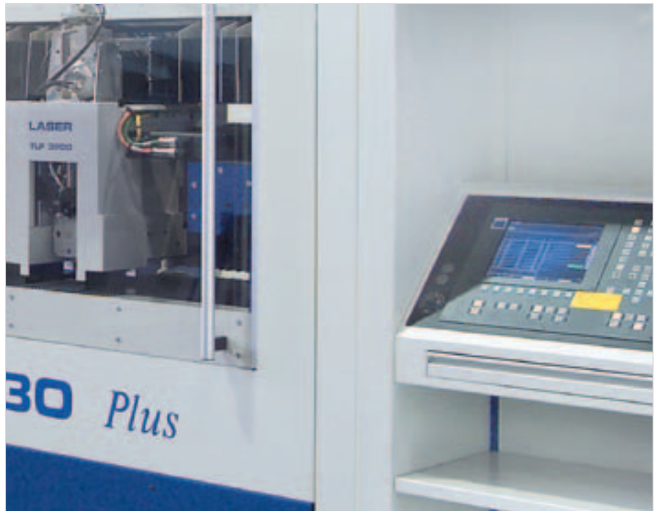
Operating panel in the machine frame
