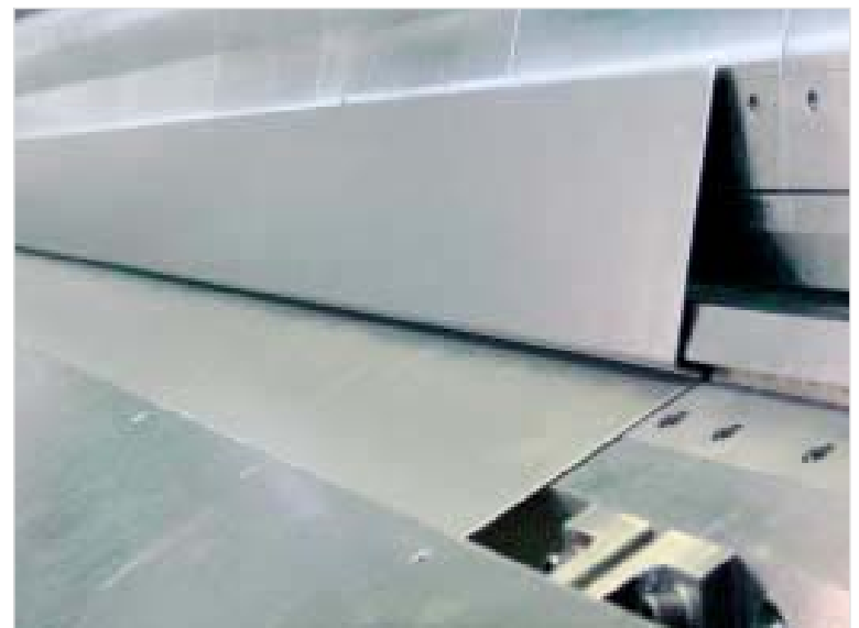
Front stop, DNC-controlled. Variable adjustment range.
