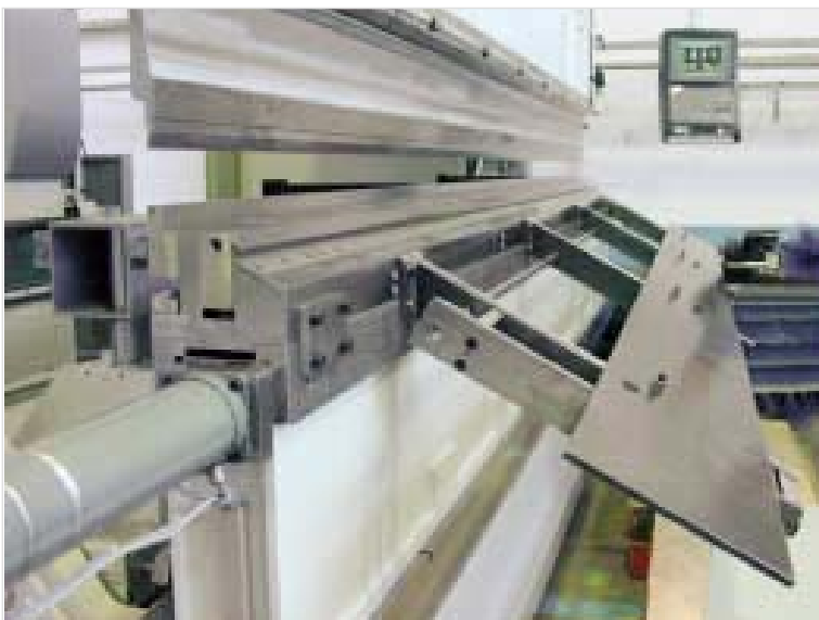
Special press brake model for producing door frames.
