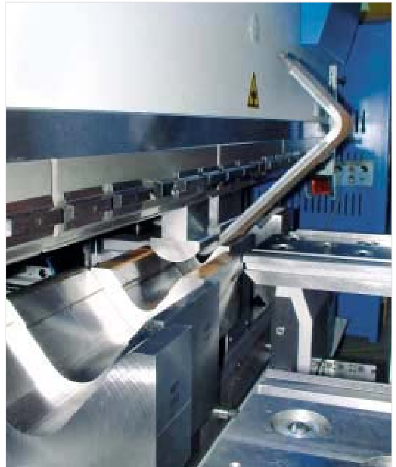
Large tool adapters for bending tasks with extreme loads.
